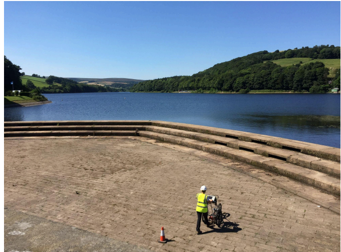
GPR Survey of Reservoir Spillway Basin
