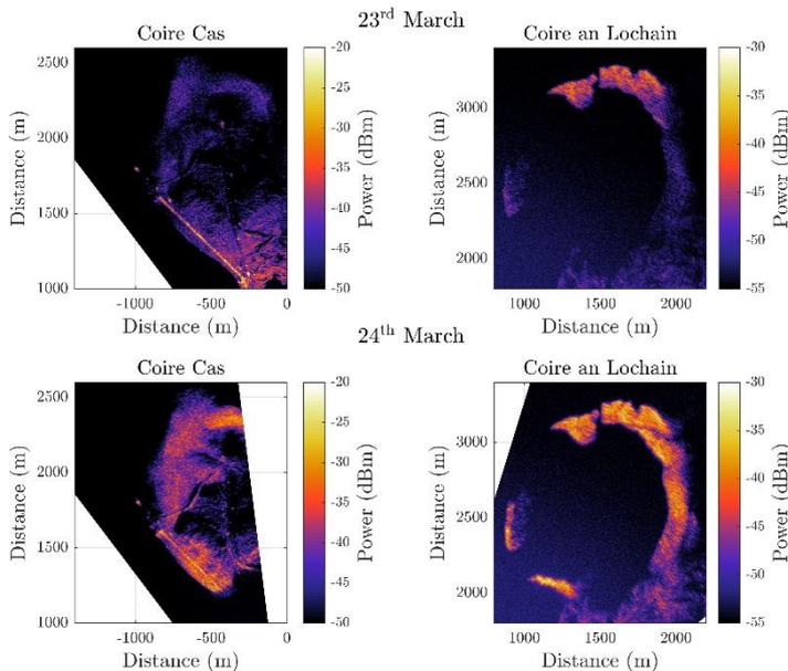
**Figure 2** Radar backscatter changes over two corries.
