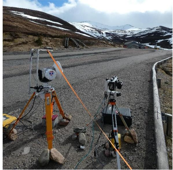
**Figure 1** Deployment of the 94 GHz radar and TLS.
